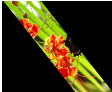
Framing Top Left X DMX value = 5 Framing Top Right X DMX value = 188 Framing Bottom Right X DMX value = 5 Framing Bottom Left X DMX value = 188 Other Framing parameter DMX values = 0
